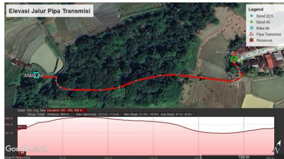
Gambar 6. Elevasi Pipa Transmisi Mata Air – Reservoir
